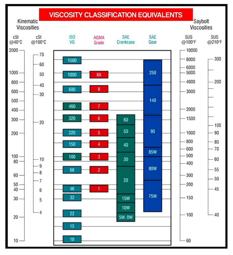
Many petroleum products are graded according to the ISO Viscosity Classification System, approved by the International Standards Organization (ISO). Each ISO viscosity grade number corresponds to the mid-point of a viscosity range expressed in centistokes (cSt) at 40° C. For example, a lubricant with an ISO grade of 32 has a viscosity within the range of 28.8 – 35.2, the midpoint of which is 32.
