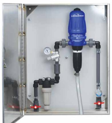
Dosatron proportional coolant mixing systems are easily installed, require no external power source and are available in a locking cabinet or easy-to-mount panel. Simply connect your water supply line driven by city water, RO, or DI water, and drop the concentrate suction hose into your barrel or tote.
